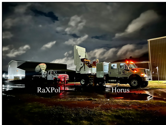
FIG. 3. Horus and RaXPol radars deployed on 8 Aug 2023, around 1039:00 UTC, to evaluate polarimetric data quality of Horus scans compared to a known reference system (RaXPol).
