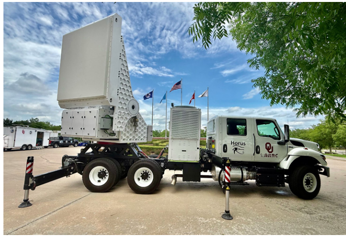
FIG. 1. The Horus fully digital S-band polarimetric PAR on its mobile platform deployed at the National Weather Center (Norman, Oklahoma).
